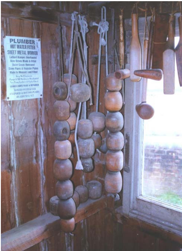
Figure 6: Bobbins used for truing bends in lead pipes. Photo: Douglas D Kent
